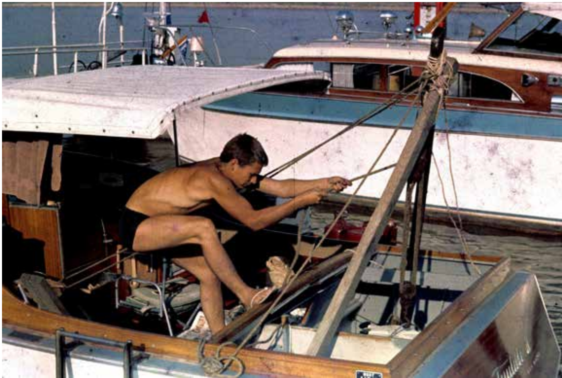
Ahde lifting the 50 HP outboard for repairs
